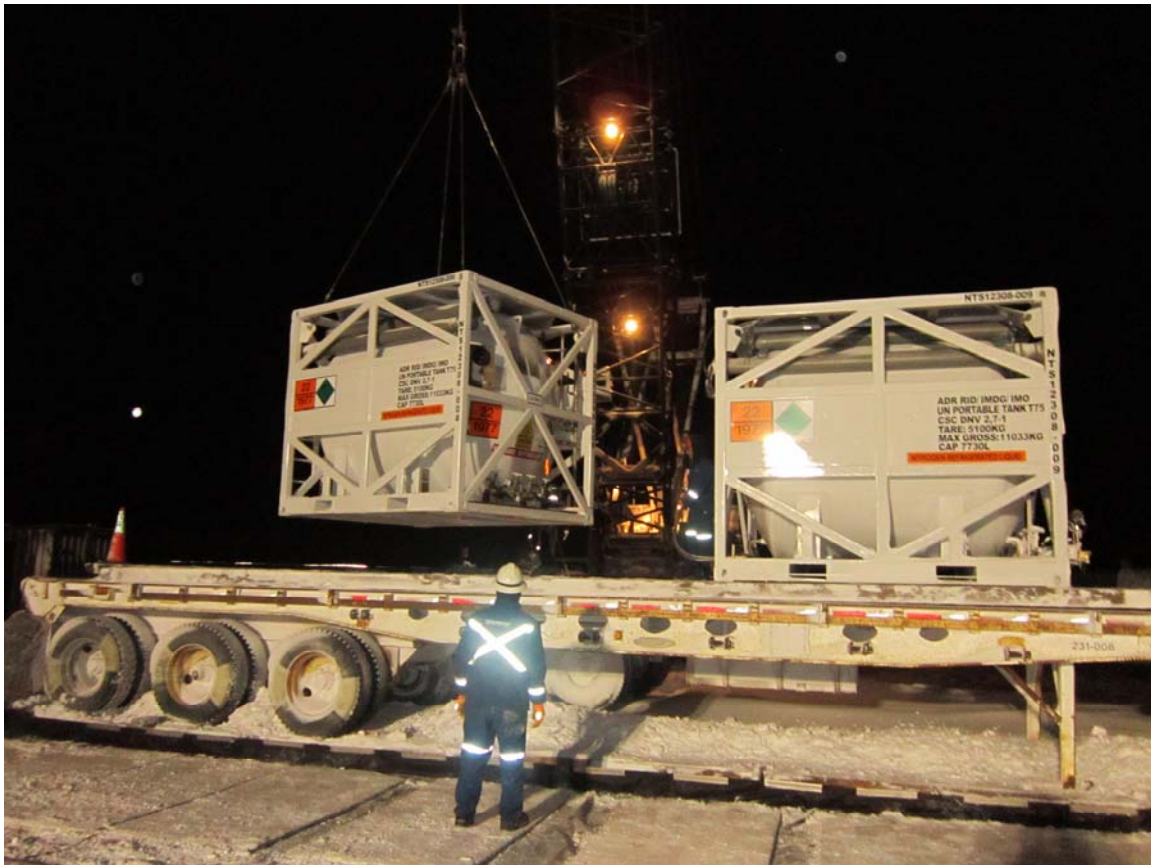
Figure 21: Spotting nitrogen tanks at Ignik Sikumi #1
