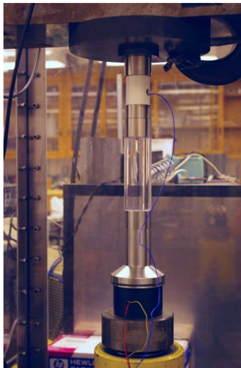
Figure 24 – Testing seismic signal quality using an acrylic core.
