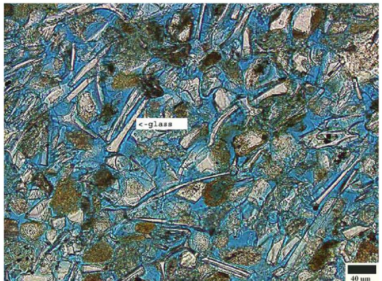
Figure 3: A side-wall core photomicrograph of porous and permeable marine sand from Alaminos Canyon block 818. This immature volcanoclastic sand contained >60% gas hydrate in situ based on log evaluation (photo courtesy of Chevron).
