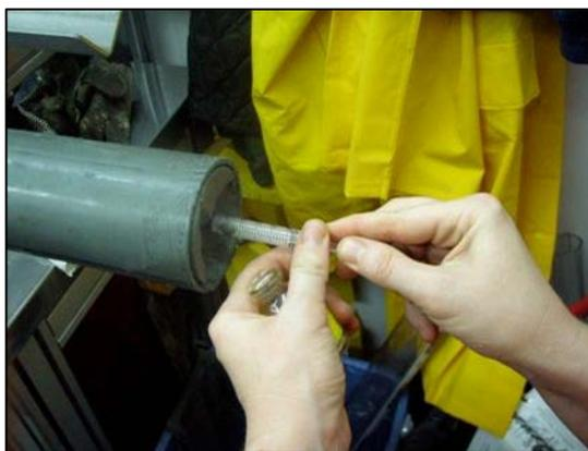
**Figure 7.6 Collecting a porewater analysis specimen.**
