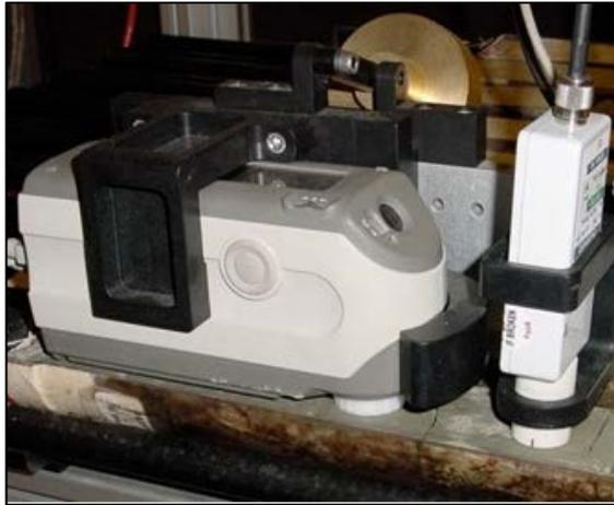
**Figure 7.12 X-ray fluorescence (XRF) spectrometer.**
