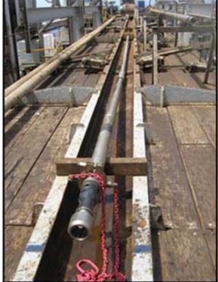
Assembly of FPC requires an open deck area of only 3 m by 12 m
