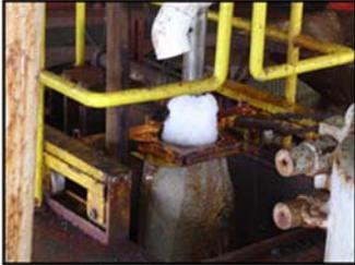
Gas Hydrate core in ice-chuck
