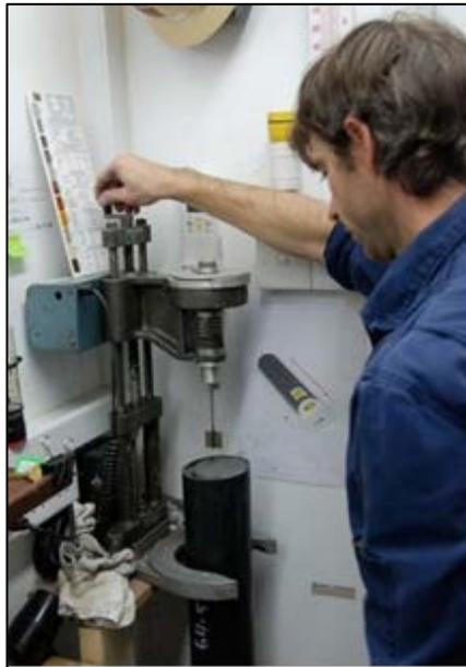
**Figure 7.7 Physical property measurement with motorized miniature vane on recovered core specimen.**
