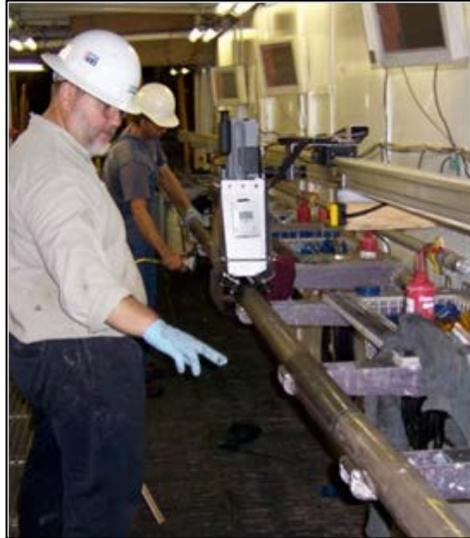
**Figure 7.2 IR scanning an APC liner on the “Catwalk” of the JR.**
