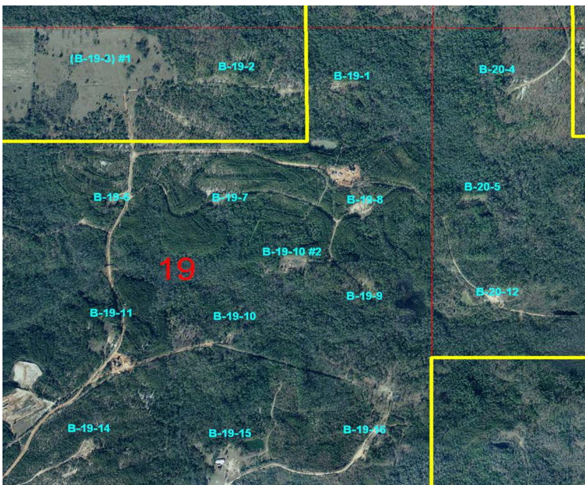
Figure 5.1. Aerial photograph of the Citronelle Oil Field in the vicinity of the test well pattern. The top edge of the photograph faces North. The test pattern consists of injector B-19-10 #2 and producers B-19-7, B-19-8, B-19-9, and B-19-11. Tank Battery B-19-8 is visible just to the Northwest of Well B-19-8. Tank Battery B-19-11 is to the South of Well B-19-11, between the roads.
