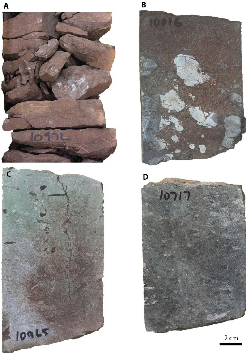
Figure 2.30. Photographs of slabbed core of the mudstone lithofacies in Well C-1-6. A. Mudstone containing pedogenic slickensides and blocky peds, 10,972 ft. B. Mudstone containing dolomitic mudstone nodules with cracks, 10,816 ft. C. Variegated sandy mudstone with desiccation crack and meniscate burrows, 10,965 ft. D. Gray mudstone with intense burrow mottling, 10,717 ft.
