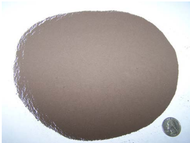
Figure 5.8. Particles of internal plastic coating and oxide scale recovered from the injector, Well B-19-10 #2, during repair of a tubing leak, separated into three size fractions. The internal plastic coating is concentrated in the largest size fraction. All of the particles, including the internal plastic coating with its attached scale, are attracted to a magnet.
