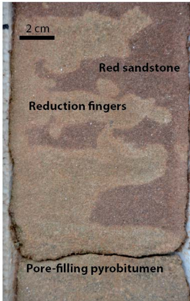
Figure 2.38. Pyrobitumen and fluid reduction fingers in Donovan sandstone showing evidence of intrusion of reducing oil-bearing fluids into red sandstone, Well D-9-8 #2, 11,139 ft.
