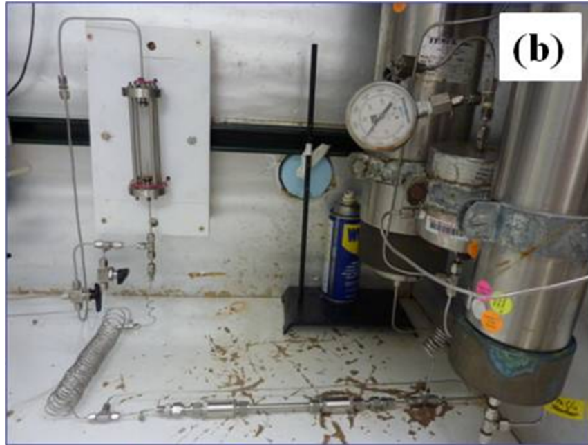
Fig. 3.2 Diagram and image of the sapphire observation tube.
