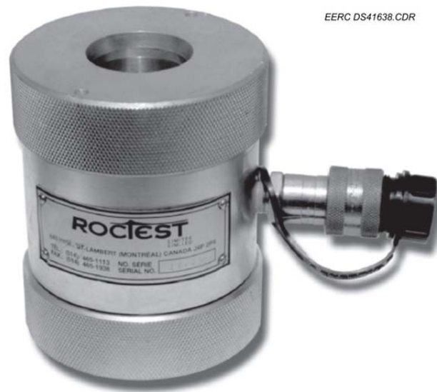
Figure A-2. Hoek cell used for applying confining pressure for triaxial testing.
