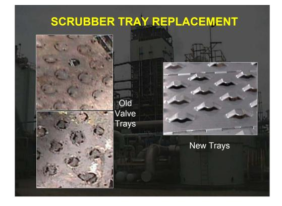
First, we are upgrading part of the syngas scrubber internals. The "polishing" section consists of trays followed by a demister. The original trays were valve type which would have been satisfactory at the design solids loading. However, since our fines production is much higher than expected, the valve caps plug and are very difficult to clean. We are replacing the trays with a new type which should perform better in this service. We are also upgrading the demister.
