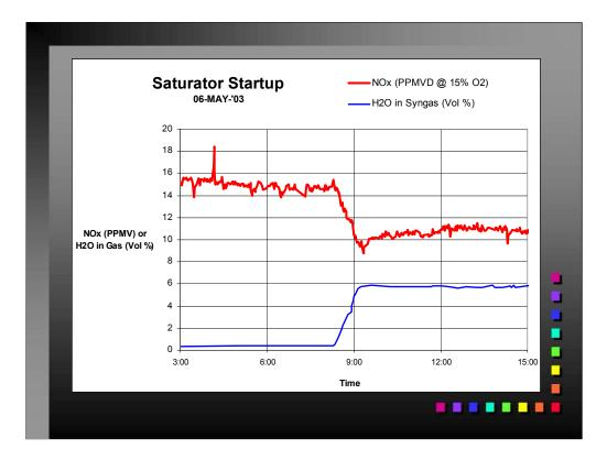
Polk was required to reduce NOx emissions from 25 to 15 ppmvd ( $15\% O_2$ ) by July, 2003. As we discussed in last year's paper, we elected to do this by supplementing diluent nitrogen with syngas saturation using low level waste heat. The system was successfully commissioned in early May. This shows the initial run. The saturator has been operating trouble-free ever since, enabling us to comply with the new permit limit.
