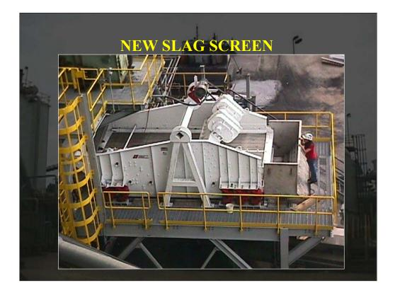
Moving forward, we are installing a new larger coarse slag screen during the current outage. It will receive our slag directly from our lockhopper and drag flight conveyor, eliminating double handling. The screen will separate the coarse, low carbon, marketable material from the fuel and fines portion. The plant is already configured to recycle this fuel and fines to slurry preparation and the coarse material can be sold with little or no post-treatment.
