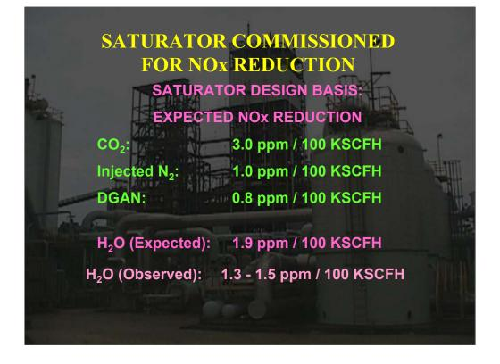
The above is the design basis we used for the saturator, I.e., we expected a 1.9 ppm reduction in NOx for every 100 KSCFH of water vapor. Although we haven't exhaustively tested the system, it appears from a few data snapshots that we only achieve about 75% of this NOx reduction. Nevertheless, this is quite enough to enable us to meet our new permit limits, and it does indicate that water vapor is significantly more effective than diluent nitrogen for NOx reduction as we expected.
