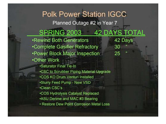
The critical path item during the spring 2003 outage was repairing the electrical insulation on both generators which took 42 days. This was the longest outage in Polk's 7 year history.
