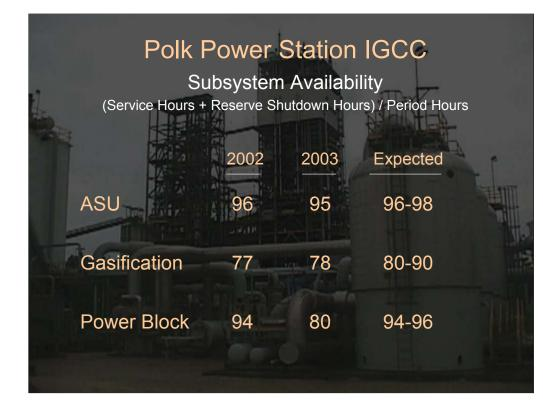
The ASU performed only slightly below its expected range, due mostly to main air compressor bearings.
