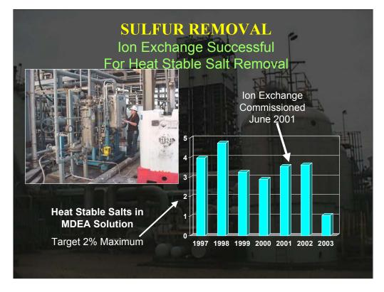
Last year, we reported commissioning our ion exchange system to remove heat stable salts from our MDEA solution. We were experiencing some accelerated corrosion in areas of the amine system that are typically vulnerable.
