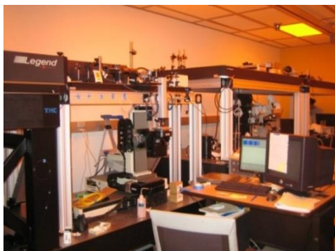
Dual-laser additive manufacturing (AM) system for fabrication of “smart parts”.
