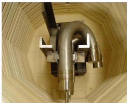
Alloy 617 in Cold Bend Test Rig.
