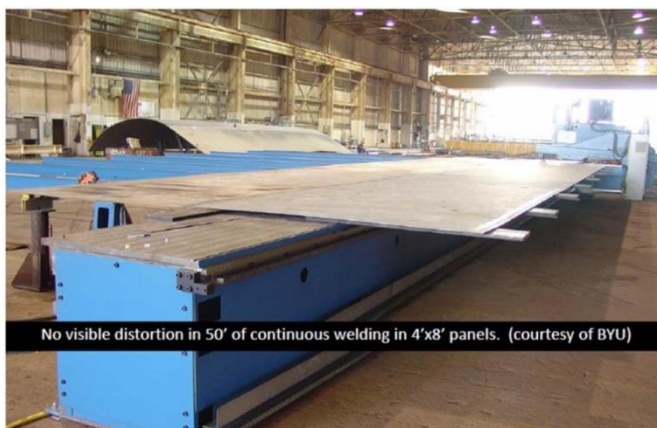
Flat plate FS welds in HSLA65 plate, stay flat.
