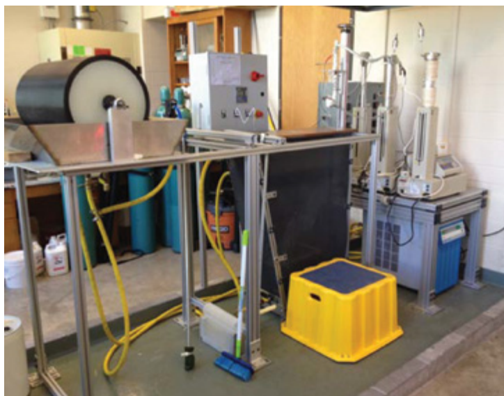
Figure 2: Georgia Tech Hollow Fiber Fabrication Line
