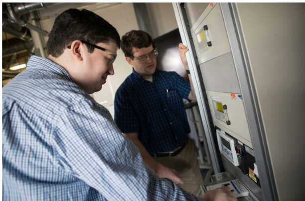
Figure 2. Researchers inspecting instrumentation measuring the outlet gas composition of the single fluid bed reactor.
