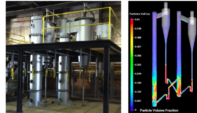
Schematic of the copper-based CLOU process, University of Utah 200 kW pilot-scale chemical looping system and simulation of the dual fluidized bed system.
