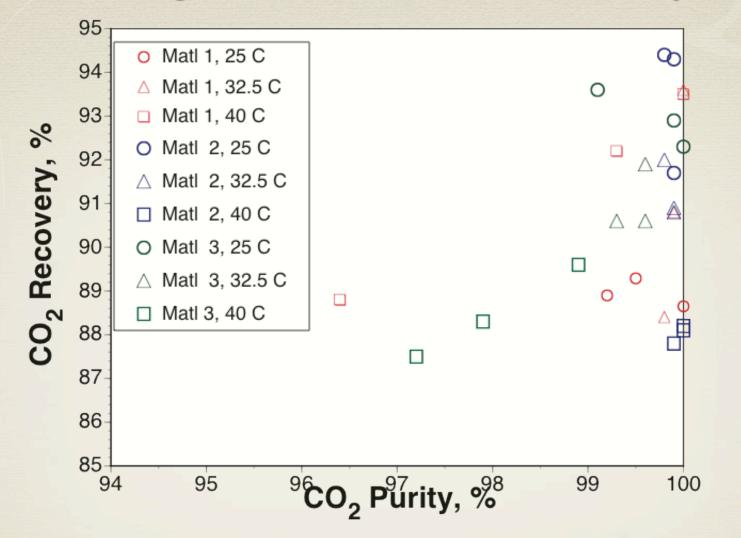
For a CO<sub>2</sub> purity of >99% and a CO<sub>2</sub> recovery of >90%, net CO<sub>2</sub> capacities of 7-9 wt% have been obtained (~15% feed CO<sub>2</sub>)
