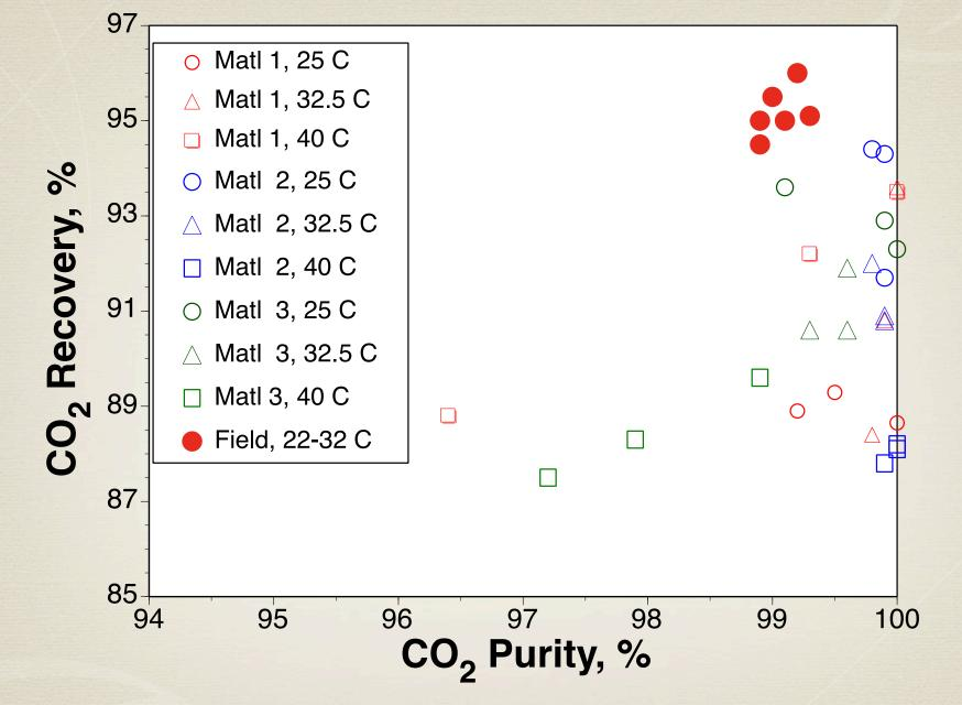
Significantly higher CO<sub>2</sub> recovery in the field compared to lab experiments
