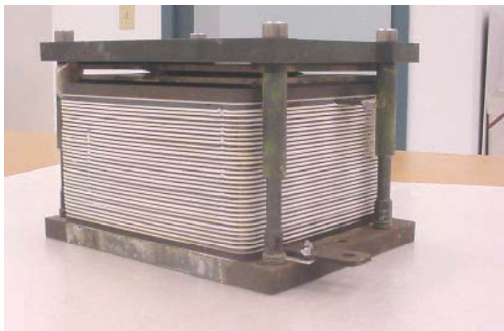
Generation 3 30-cell stack (3.5 liter, 13 Kg)
