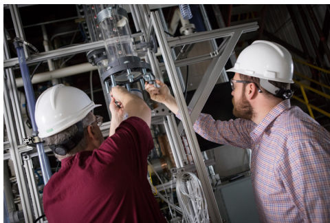
Figure 7. Researchers assembling the cold-flow carbon stripper.
