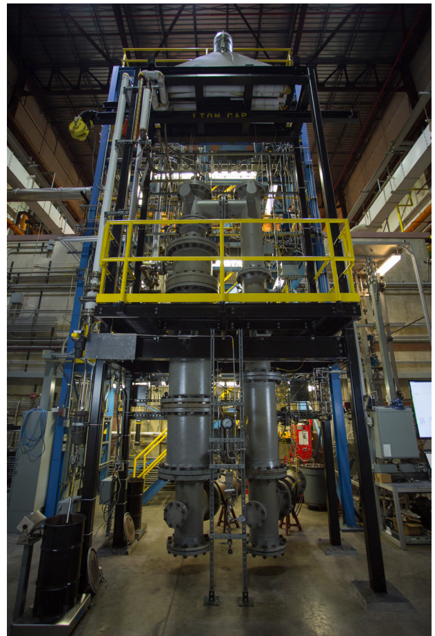
Figure 4. 50-kWth chemical looping reactor.
