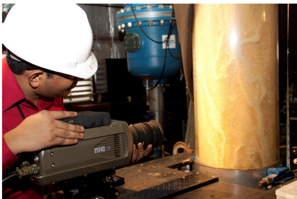
Figure 3. Researcher collecting high-speed video for particle tracking.
