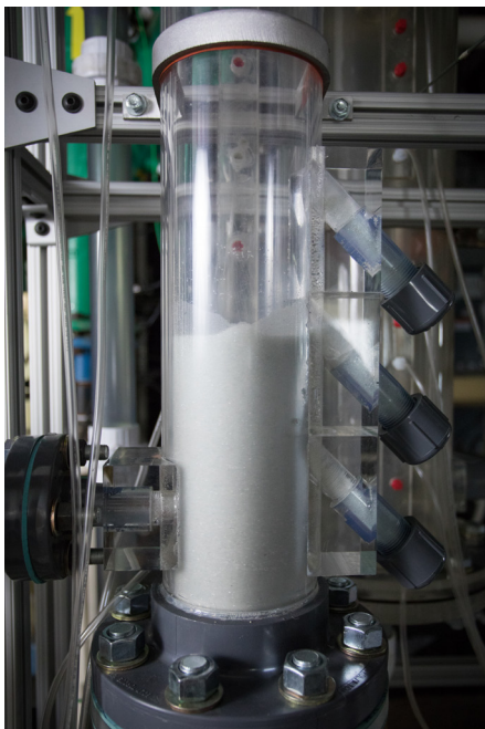
Figure 5. 4-inch diameter cold-flow bubbling fluidized bed.
