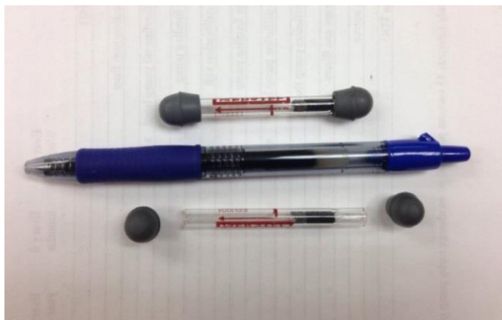
Figure 4. Glass tubes filled with Ambersorb® carbonaceous polymer adsorbent (pen for scale).
