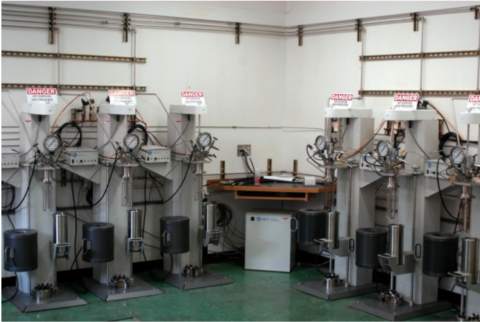
Figure 1. Six fixed-head autoclave system with PC interface.
