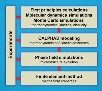
Multi-scale materials simulations supported by critical experiments.
