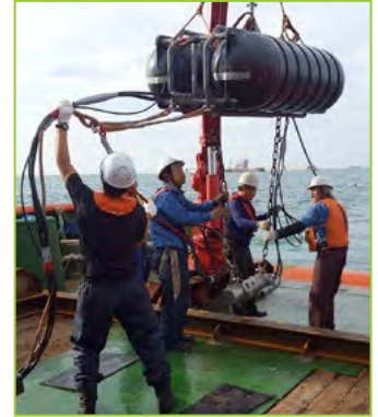
Acoustic energy sources (compressed air) being deployed for ultra-high-resolution 3D seismic data acquisition at the Tomakomai CO 2 storage demonstration project offshore Tomakomai, Hokkaido, Japan.
