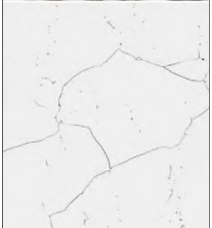
Microstructure of Haynes 282 alloy as-cast (top) and homogenized (bottom).
