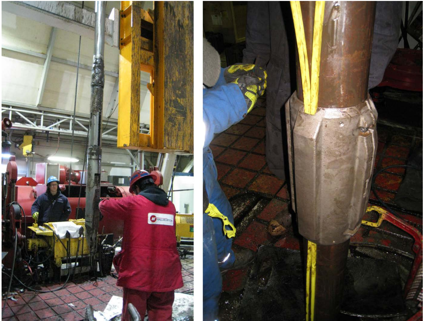
Figure 4. Data acquisition activities at the Hydrate-01 well included CoreVault™ side-wall pressure coring (left) and deployment of twin DAS/DTS fiber-optic cables as strapped to the well casing during completion (right).
