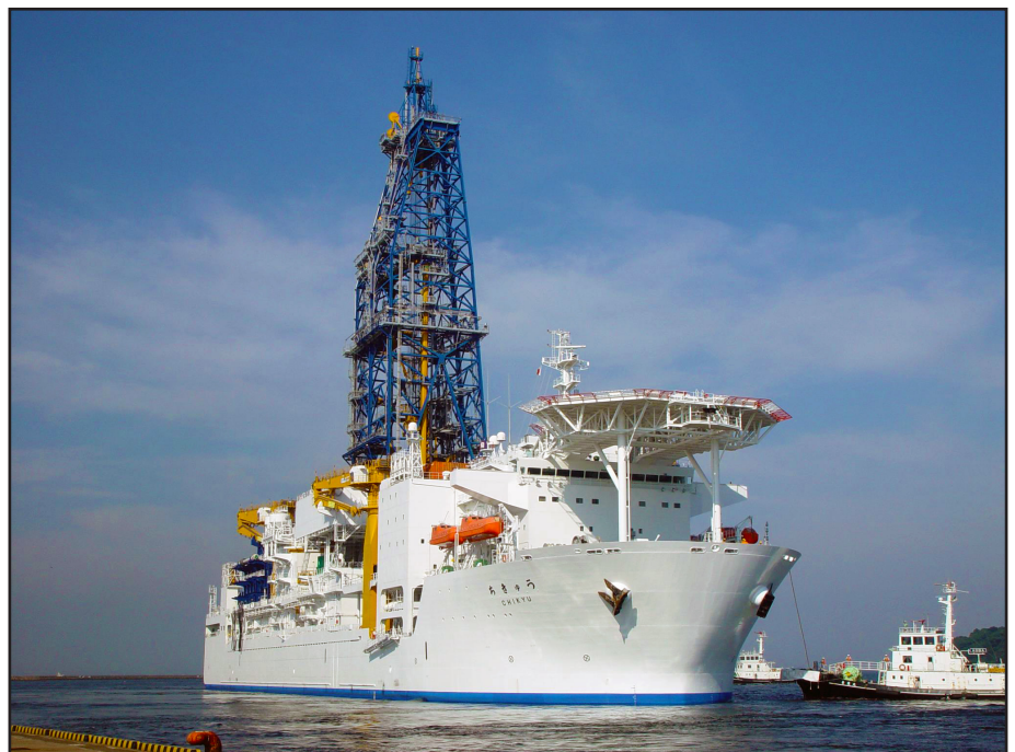
Figure 1. The deepwater D/S Chikyu, as deployed during NGHP-02, was designed by the Japanese government for international scientific drilling operations.
