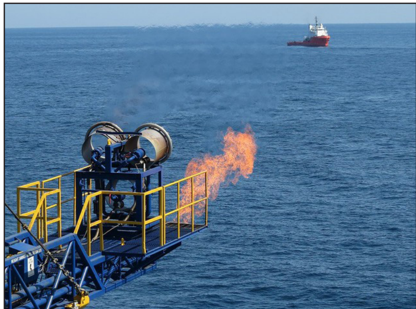
Figure 1. Methane gas flare resulting from methane hydrate de-pressurization test, Daini Atsumi Knoll, eastern Nankai Trough, Japan. Photo credit: JOGMEC
