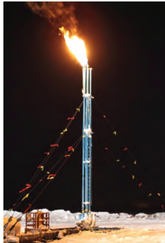
Figure 2: After measurement and compositional analysis, gas is flared at the Iġnik Sikumi # 1 well site.
