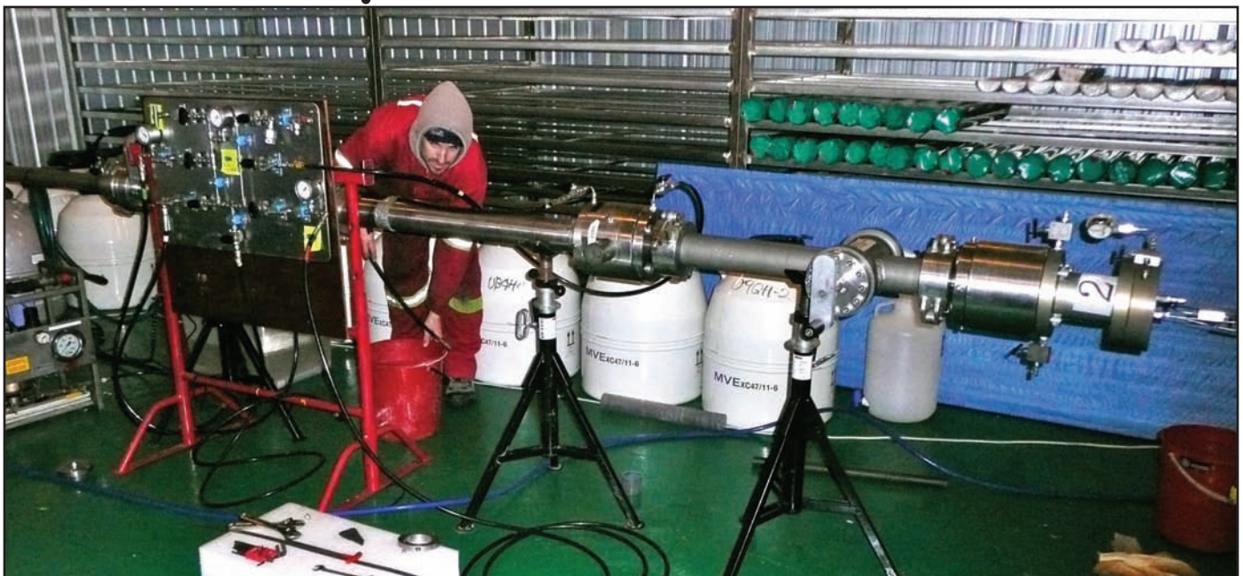
Figure 1. The core cutting sub components of PCATS connected to the effective stress cell ready for sample cutting and transfer.
