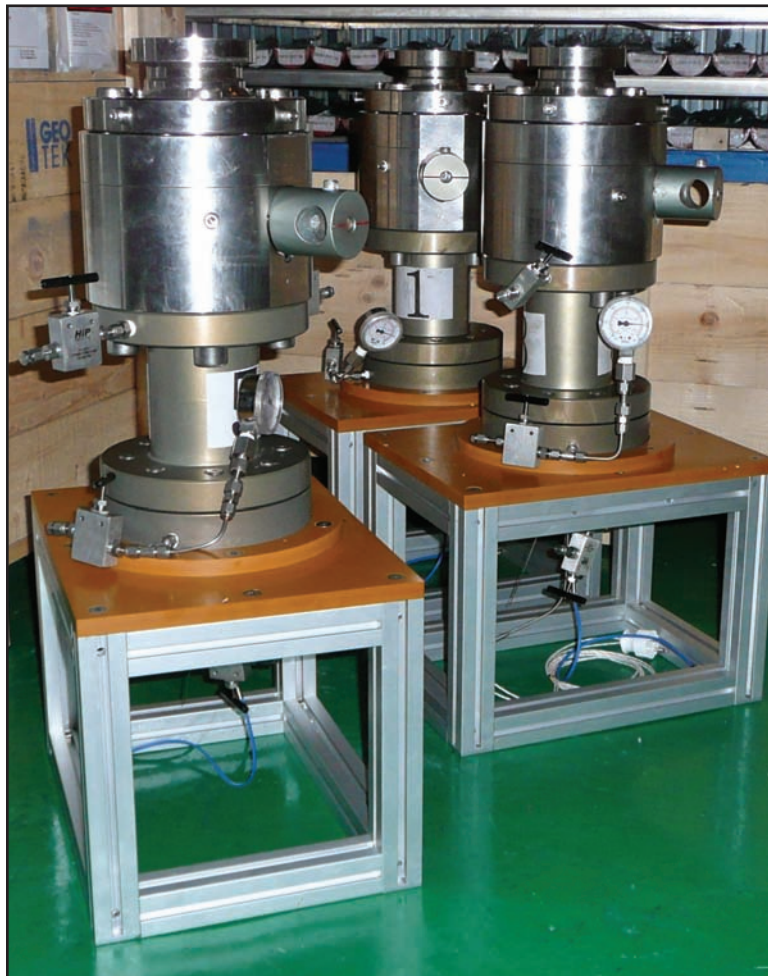
• Figure 2. Three of the five GHOBS containing the pressurized • sub-samples ready for testing.
