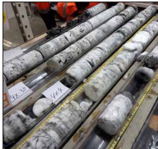
Figure 7. Thick, massive hydrates recovered from 17 mbsf at Site J20, about 150 meters northwest of Site J24. Pure hydrate cores were X-ray CT scanned and dissociated onboard to recover hydrate gases, hydrate water, and insoluble residues in the hydrates. Samples were then stored in liquid nitrogen.
