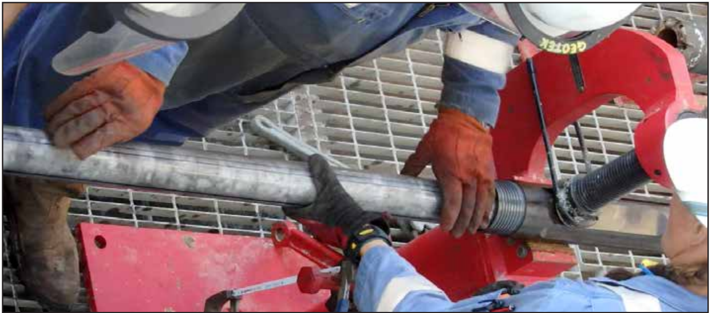
Figure 6. Coring operation for the 2015 campaign was conducted by GeoTek Ltd. The photo shows the recovery of hydrate on deck from about 22 mbsf at Site J24.
