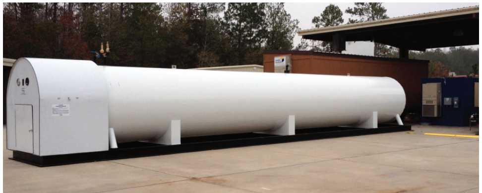
L&S Cryogenics recently completed fabrication of the CO 2 tank (in white) and the gas mixing skid (in blue) that will be used during the field test.
