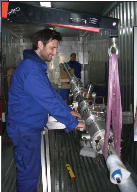
Subsectioning pressure cores with the PRESS system.
