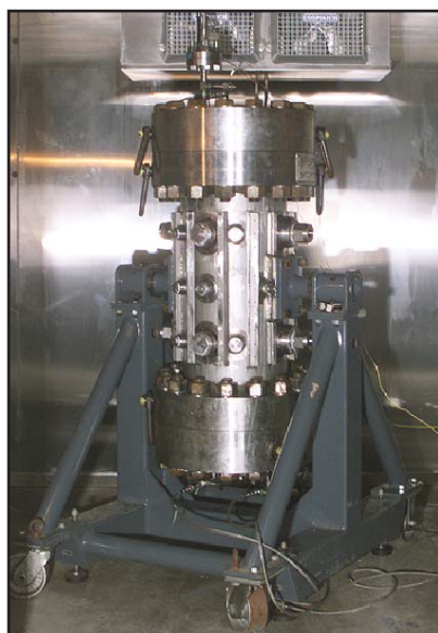
Figure 1: ORNL's 72-liter SPS is designed to conduct meso-scale gas hydrate accumulation and dissociation studies.
