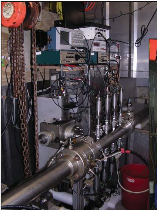
Experimental set-up for obtaining measurements using the IPTC.
