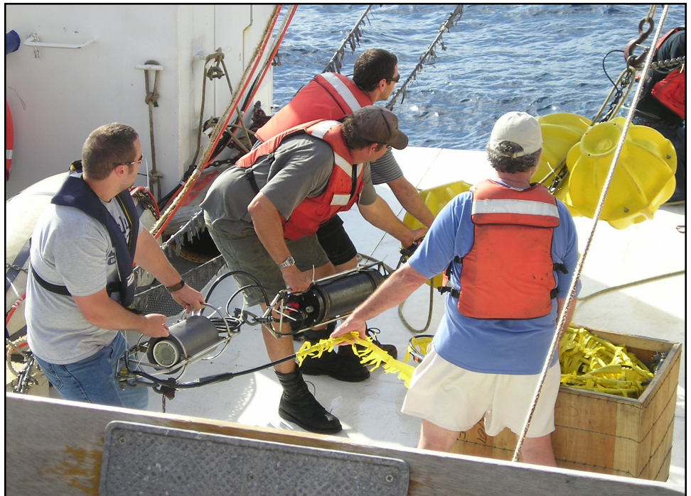
A prototype of the vertical acoustic array was tested in 2002 using a watergun energy source.
