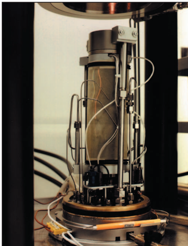
Close-up view of a test specimen about to be raised into the main pressure vessel (visible at the top of the photograph).
