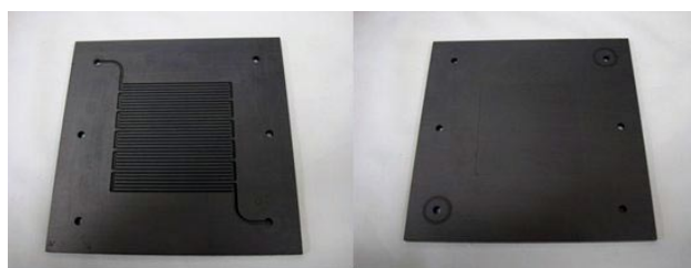
FIGURE 4. Photographs of a cathode current collector plate showing three-channel serpentine flow field (left) and flat surface for electrical connection to anode composite plate (right)
