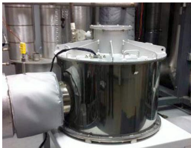
FIGURE 4. 3–5 kW module integrated into the modified 30 kW test facility
