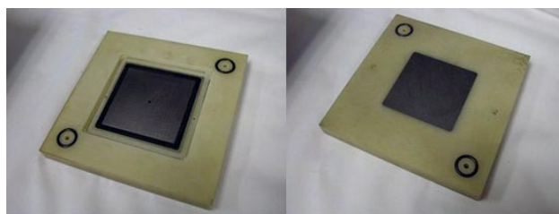
FIGURE 3. Photographs of a composite anode plate showing one side machined to mate with porous IFDL plate and sealing gasket (left) and flat surface to allow electrical contact with cathode current collector (right)
