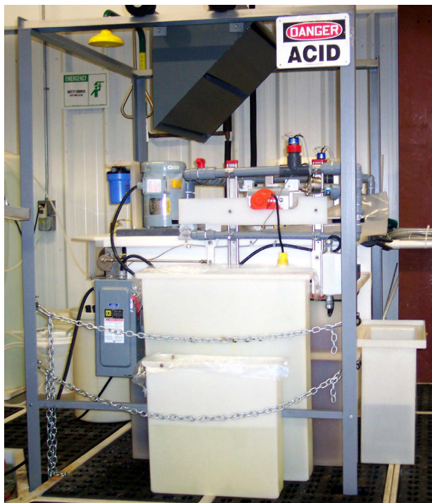
FIGURE 3. Photograph of Modified FARADAYIC Electrodeposition Cell for Mn-Co Alloy Deposition onto SOFC Interconnects
