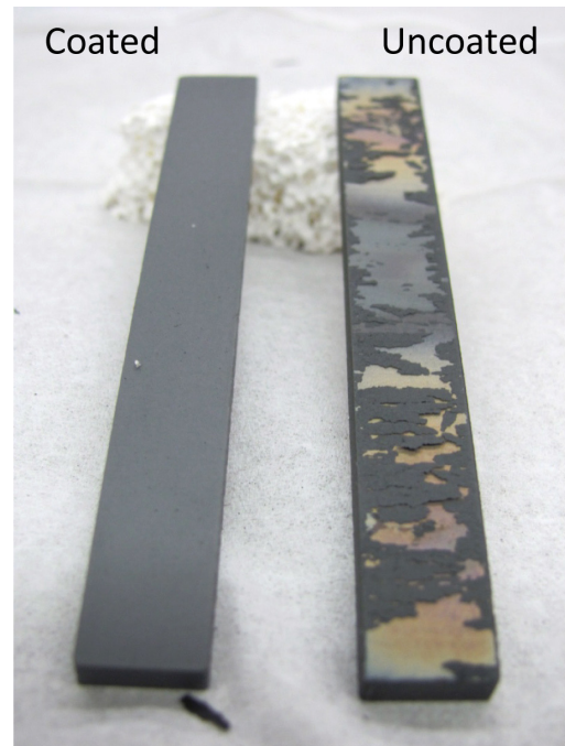
FIGURE 5. Coated and Uncoated AL SS441 Substrates after Accelerated Oxidation at 900°C for 200 Hours in Air
