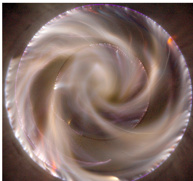
FIGURE 2. An Image of Gliding Arc Plasma as Taken from the Reactor Installed at NETL
