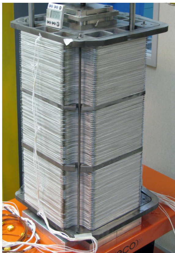
FIGURE 2. 92-Cell SOFC Stack Block
