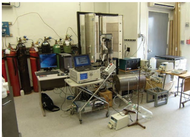
FIGURE 1. Experimental Set-up for 30-Cell Delphi Stack with System Components
