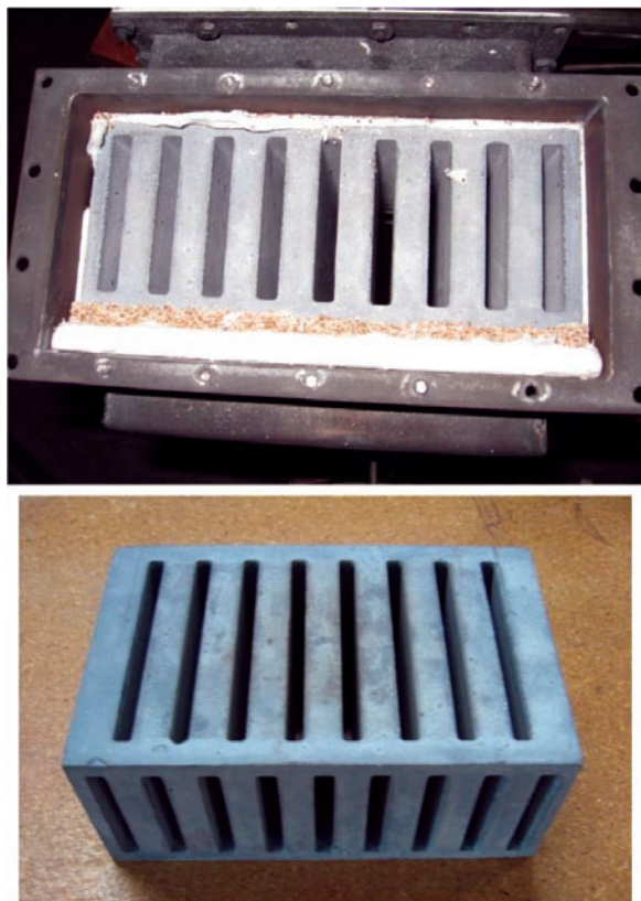
FIGURE 4. 6.3 mm Ceramic Core after 1,000 Hours of Operation
