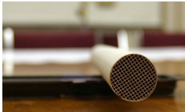
FIGURE 3. Alumina Monolith Coated with NETL Reforming Catalyst, Prepared by Nextech
