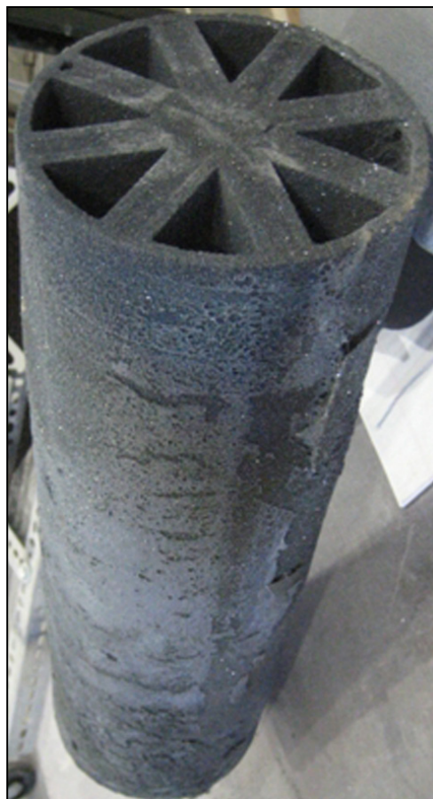
FIGURE 1. Prototype Heat Exchanger
