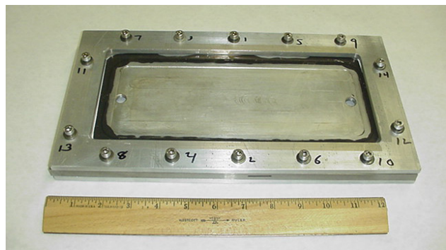
FIGURE 2. Parallel-Plate Dielectric Barrier Discharge Device
