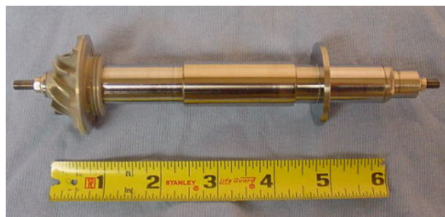
FIGURE 3. FPS Blower Rotating Assembly
