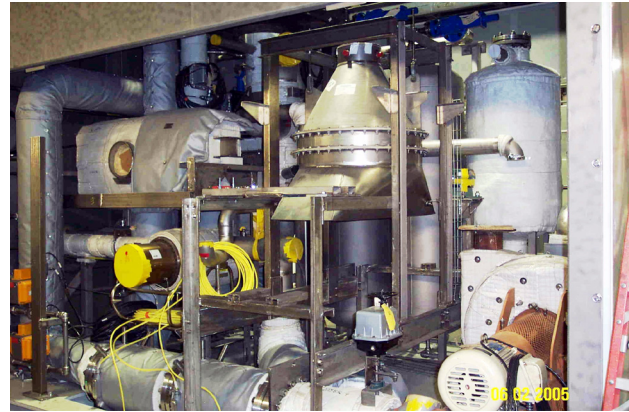
Figure 4. Fabrication of Alpha Unit in a Packaged Sub-MW Class Hybrid Power Plant Configuration
