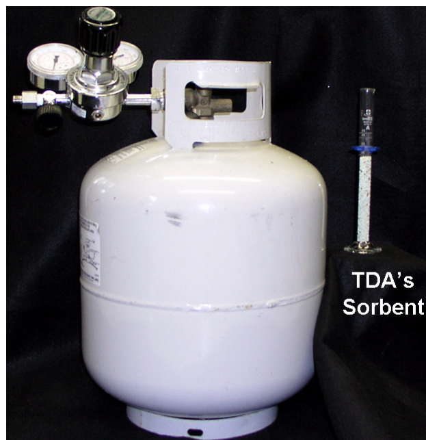
Figure 4. TDA's LPG Desulfurization Sorbent
