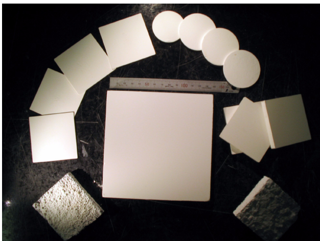
Figure 3. CERCANAM Insulation Materials Fabricated in Various Shapes and Sizes
