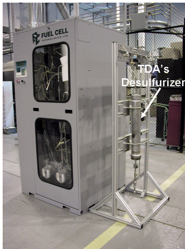
Figure 3. TDA's Desulfurizer in Combination with SWPC's 5 kW e SOFC during Alpha Testing
