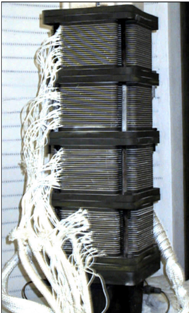
Figure 3. KW-class SOFC Stack Tower: The internally manifolds 80-cell stack tower produced 3.5 kW.
