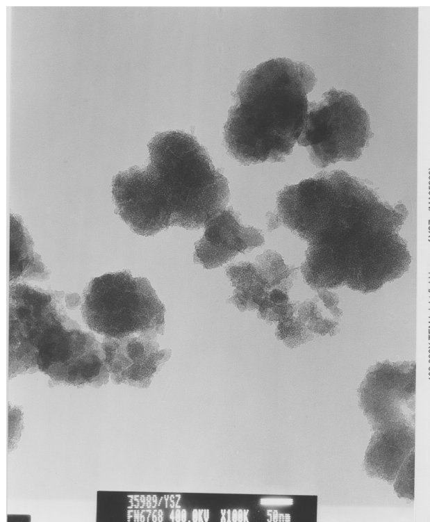
Figure 2. A bright field TEM image of nanosize YSZ formed by the MD process. The crystallite size is ~5 nm. The agglomerate size in this TEM image is about 50 to 200 nm. The agglomerates are soft and can be broken with ease, down to a few tens of nm.
