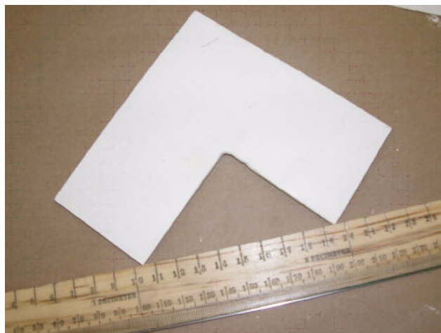
Figure 1. An L-shaped CERCANAM Specimen That Showed No Significant Damage after 9 Thermal Cycles from Room Temperature to 850°C, Followed by an Aggressive Thermal Shock Test
