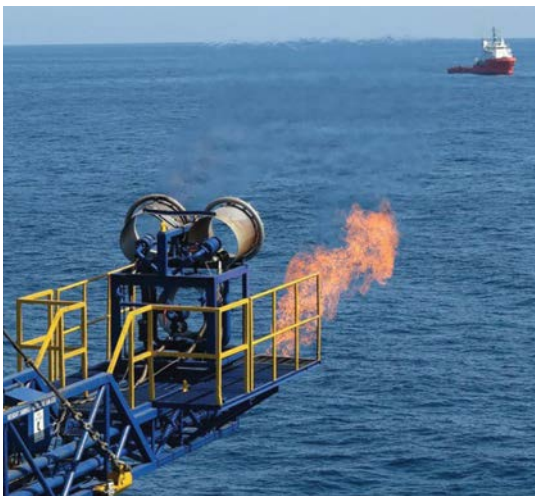
Methane gas flare resulting from methane hydrate depressurization test, Daini Atsumi Knoll, eastern Nankai Trough, Japan. Photo credit: JOGMEC.
