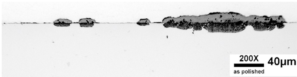
TP347HFG, 500h at 700°C & 200 bar CO 2 (Pint & Keiser, 2014)
