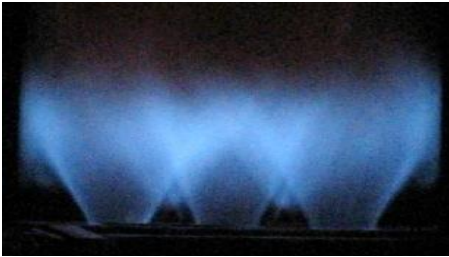
Line-of-sight photograph of multi-nozzle flame
