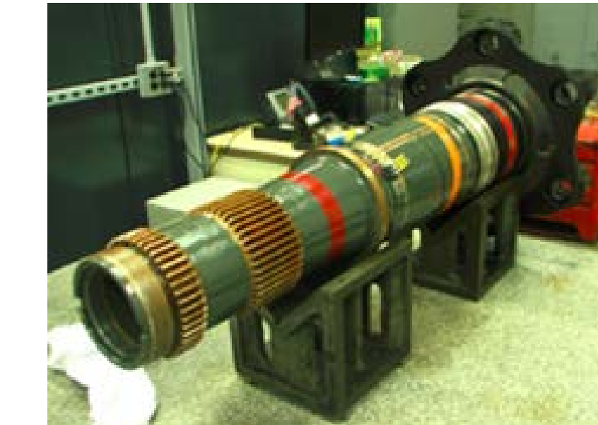
Ferrium C61™ rotor shaft for Boeing Chinook helicopter offers 20% increase in power density (power to weight ratio) versus incumbent steel
