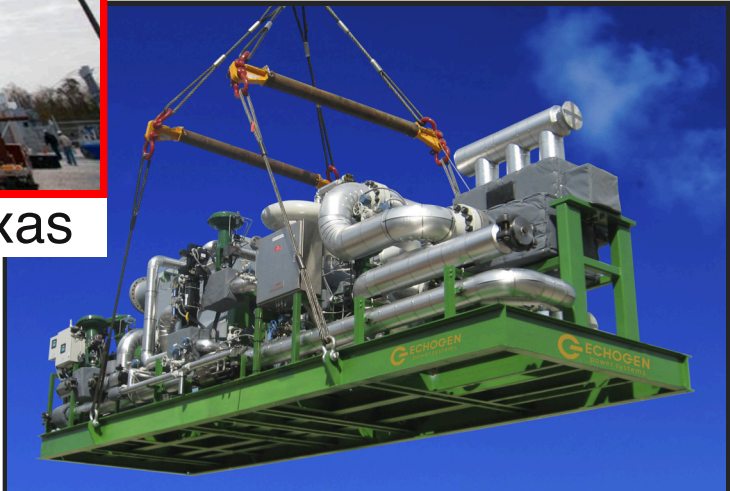
7MW Echogen, waste heat
