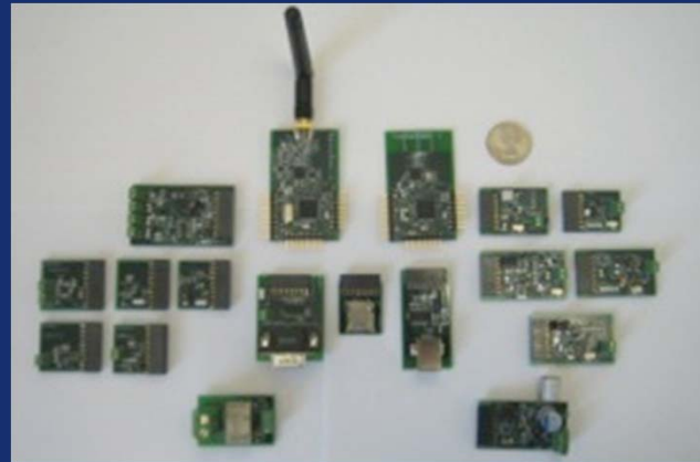
NanoSonic's Wireless Sensor Modular Hardware, "M" Shape Antenna Operates at 2.4 GHz band with 25 Possible Channels
