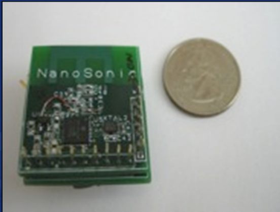
NanoSonic's Wireless Sensor Modular Hardware, "M" Shape Antenna Operates at 2.4 GHz band with 25 Possible Channels
