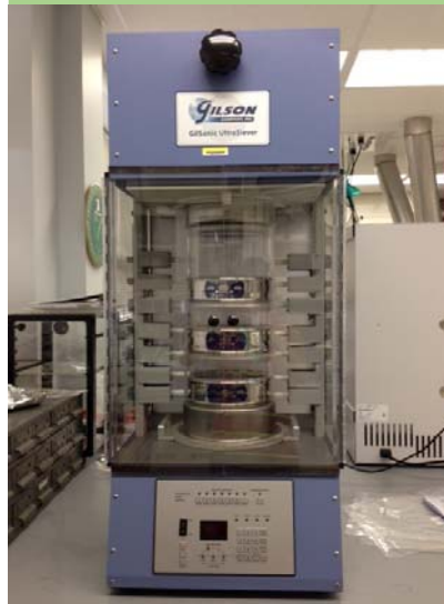
Ultrasound Shaker Sieve size down to 5 micron
