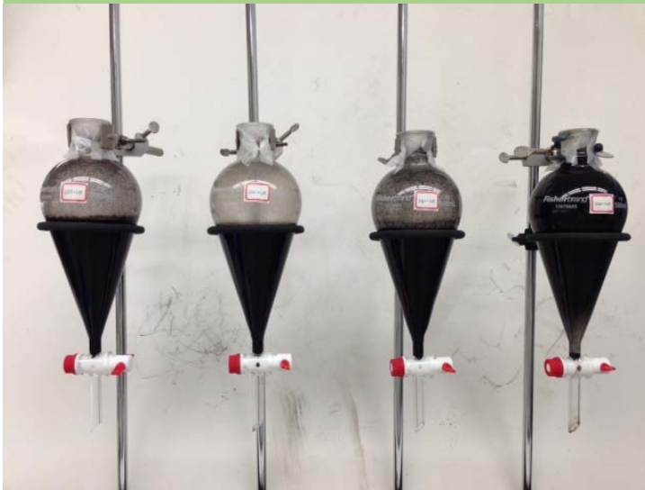
Float-sink separation Bottom dense fraction
