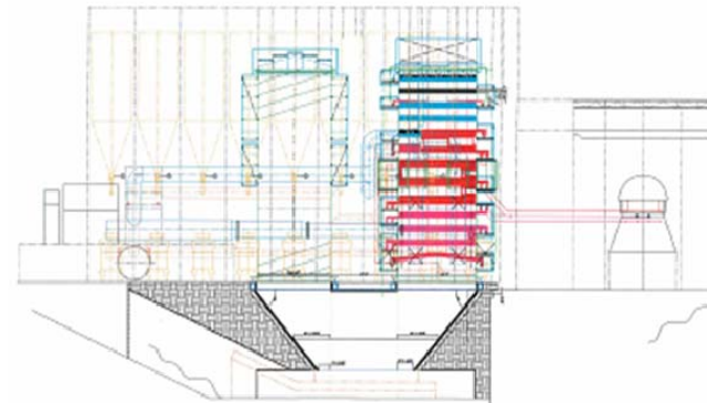
Downdraft Inverted Tower Boiler*
