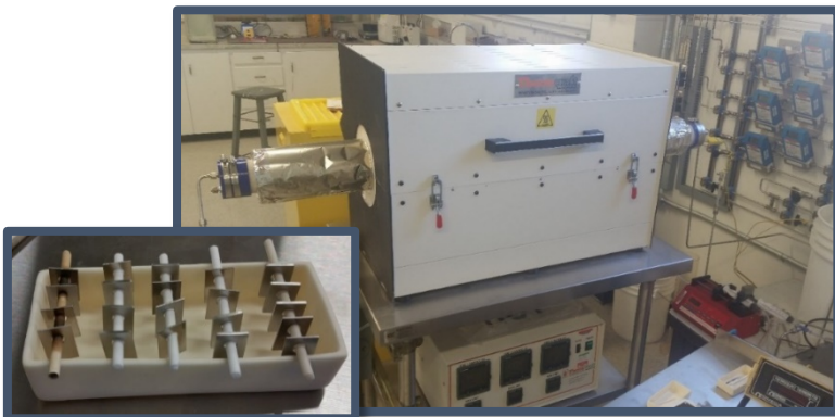
Tube furnaces for ambient pressure exposures
