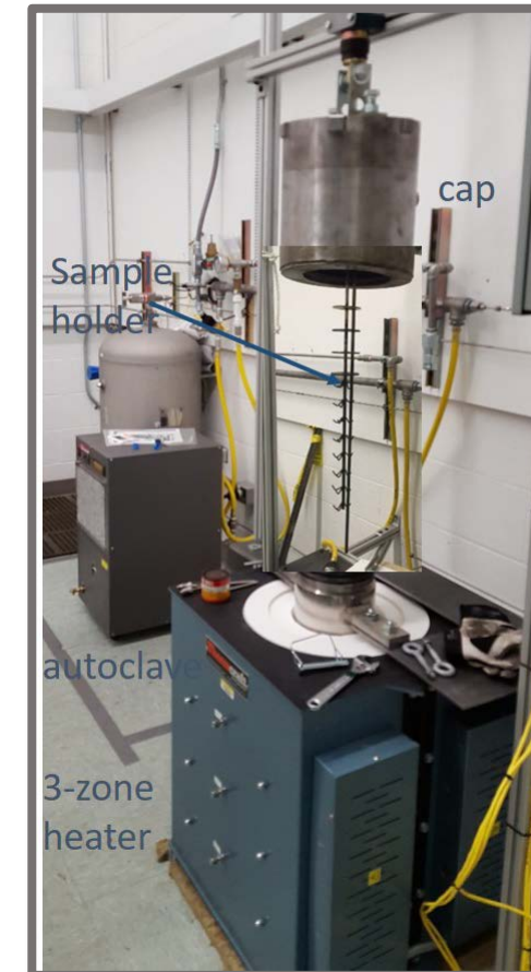
CO 2 Autoclave designed for 275 bar CO 2 at 800°C. Capable of injecting H 2 O as an impurity.
