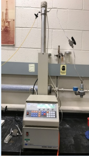
CO 2 delivery pump
