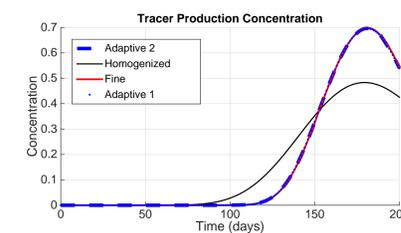
Figure 2: Tracer concentration history at production well for a homogeneous permeability distribution of 50 mD
