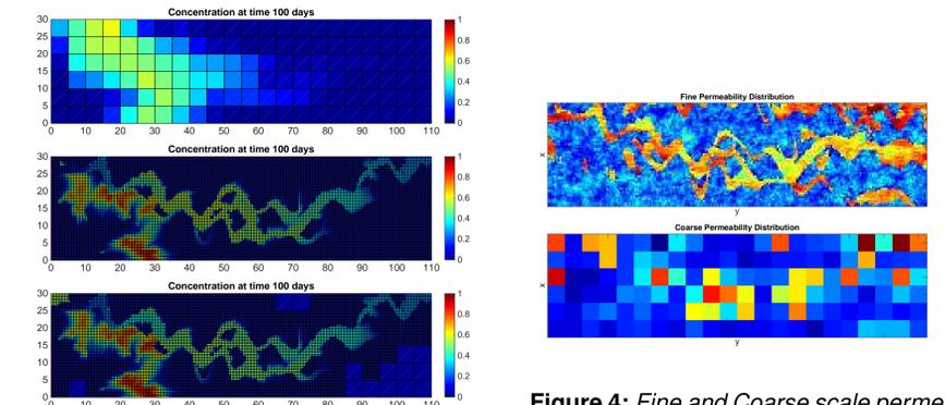
Figure 3: Concentration profiles at 100 days for coarse (top), fine (middle) and adaptive (bottom) approaches
