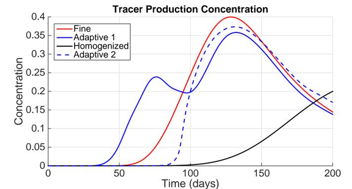
Figure 5: Tracer concentration history at the production well for SPE layer 37.
