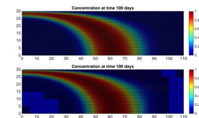
Figure 1: Concentration profiles at 100 days for fine (top) and adaptive (bottom) approaches
