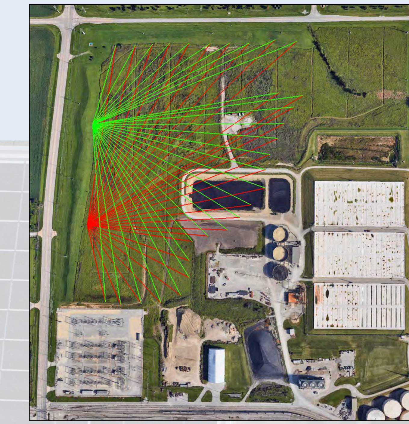
Figure 3. (a) Site layout showing chords from transceivers (T1 and T2) to reflectors. (b) 2-D recreation of the atmospheric CO 2 concentrations collected from the GreenLITE system.
