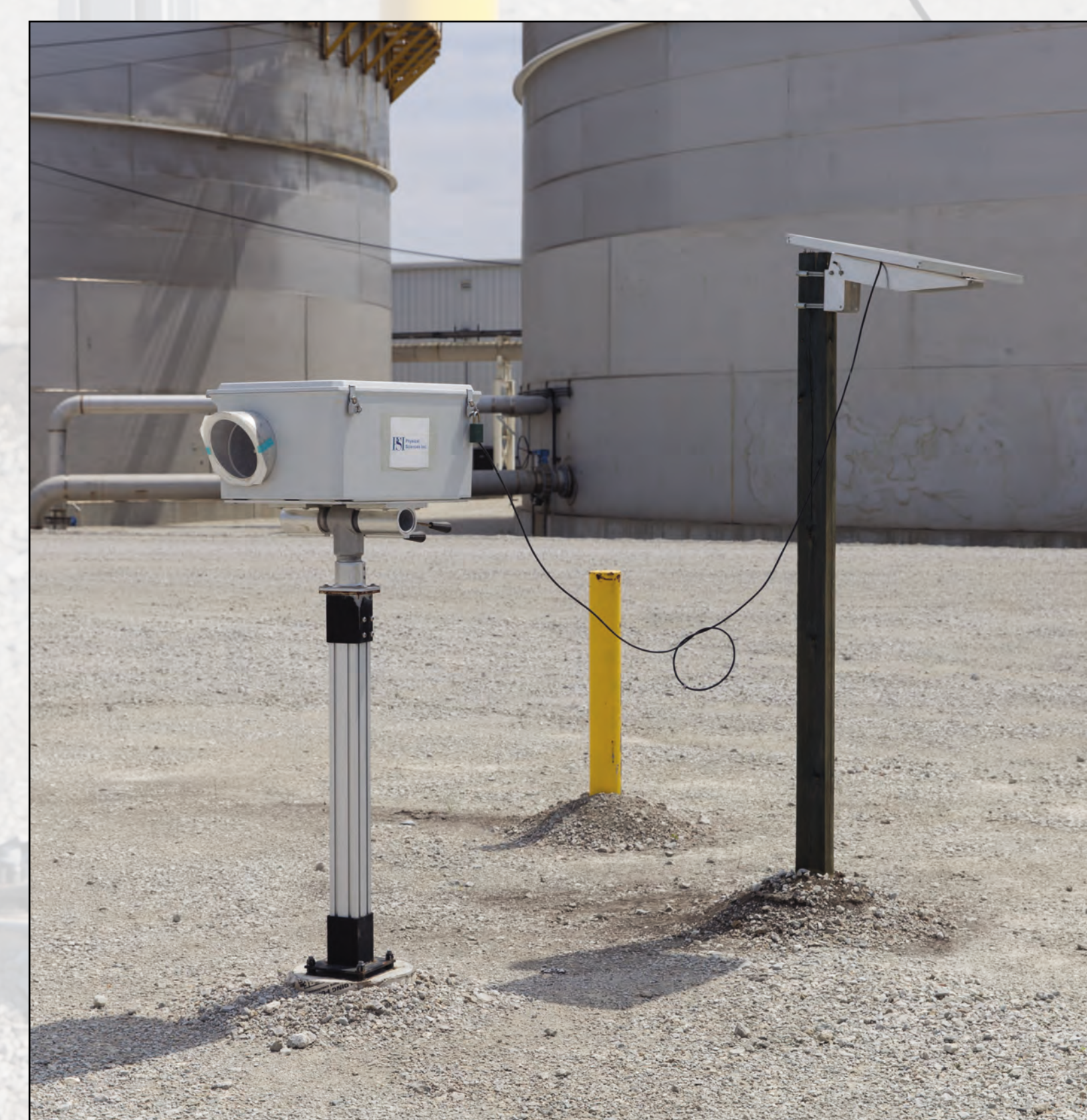
Figure 1. Prototype CO 2 Open-Path Sensor (OPS) installation at IBDP CO 2 injection wellhead in Decatur, Illinois: (a) aerial view of IBDP injection site, and (b) OPS transceiver with solar panel supply.
