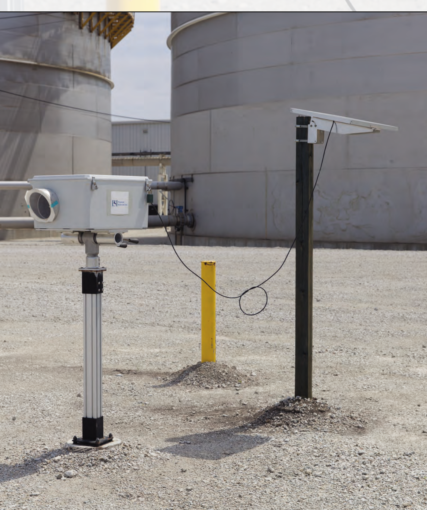
Figure 1. Prototype CO 2 Open-Path Sensor (OPS) installation at IBDP CO 2 injection wellhead in Decatur, Illinois: (a) aerial view of IBDP injection site, and (b) OPS transceiver with solar panel supply.
