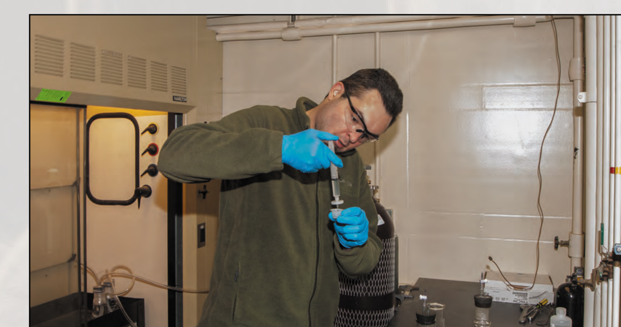
Figure 3. Samples were collected periodically by syringe, filtered, and acidified prior to analysis.
