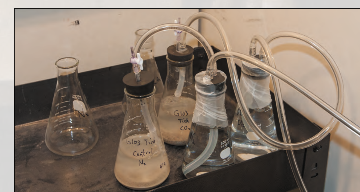
Figure 2. The batch set-up involved a water-rock ratio of 3:1. Both N 2 and CO 2 flowed through separate flasks of deionized water to saturate each gas with water and prevent evaporation.
